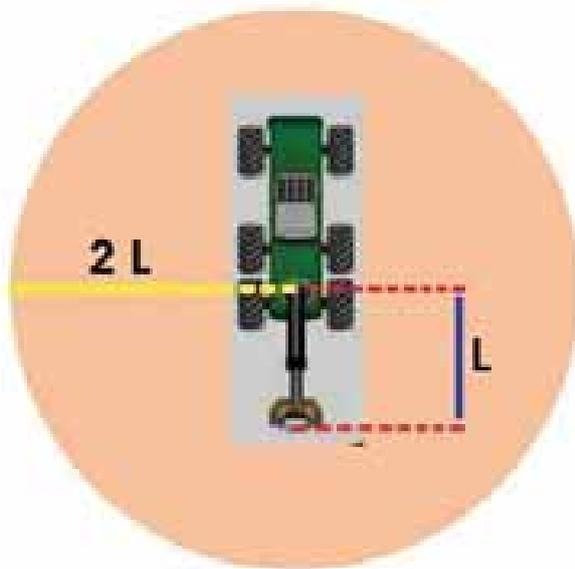
Figure 7. The orange area shows the danger area corresponding to the range of action (L) of the hydraulic arm.
