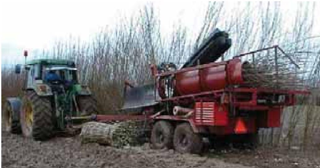
Photo 41. Trailer mounted harvester unloading the bale along the road.
