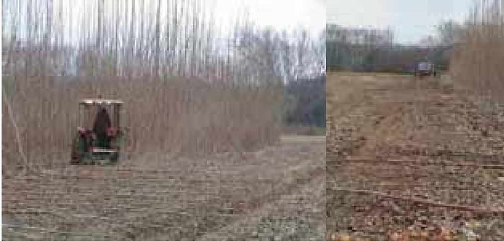
Photo 40. A simple harvester, based on a circular saw, cuts the trees and pushes them by the side. Following a tractor with a special front end loader piles them up to the field headland for stocking or chipping.
