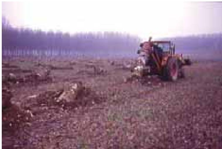
Photo 37. A farm tractor mounted auger extractor at work on a poplar plantation.
