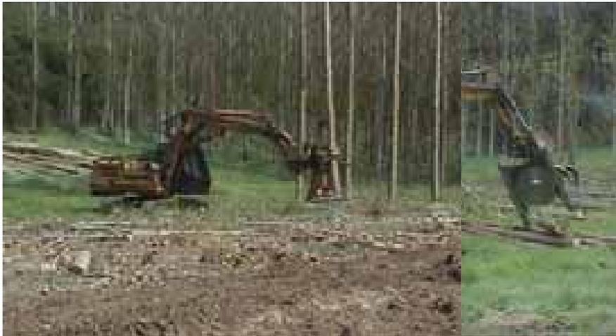
Photo 7. Felling by disc head on an excavator, in the advanced mechanization.
