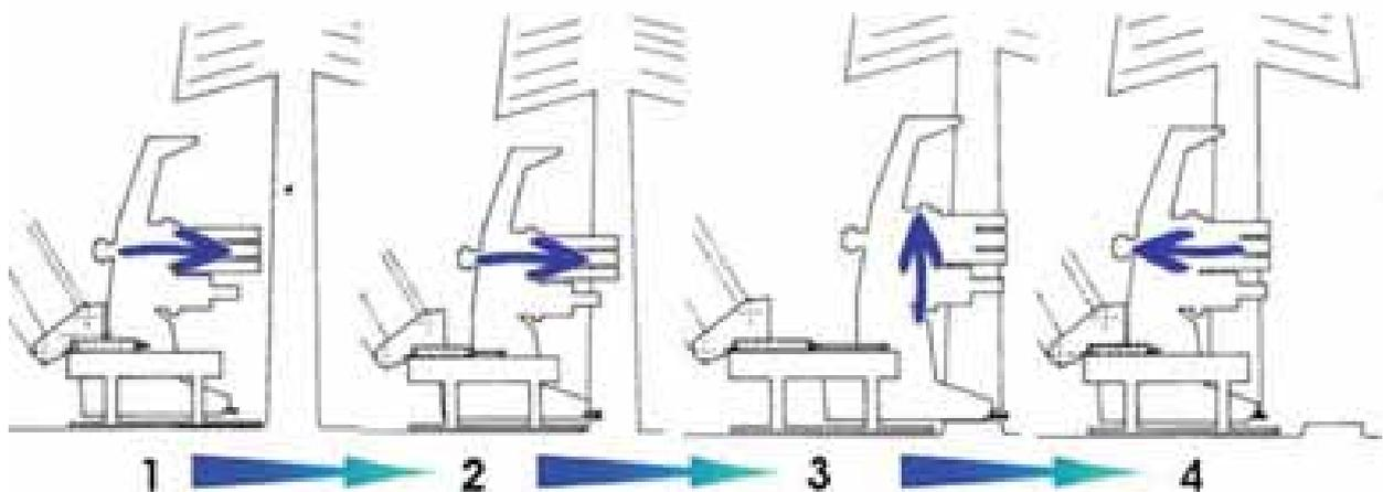
Figure 5. Sequential diagram of felling with felling head: the arrows indicate the movement of the head.
