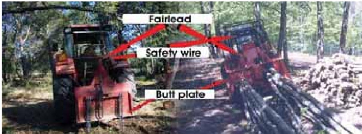
Photo 18. On the left a forest winch with one drum and on the right with two drums; both forest winches are of mobile or carried type.
