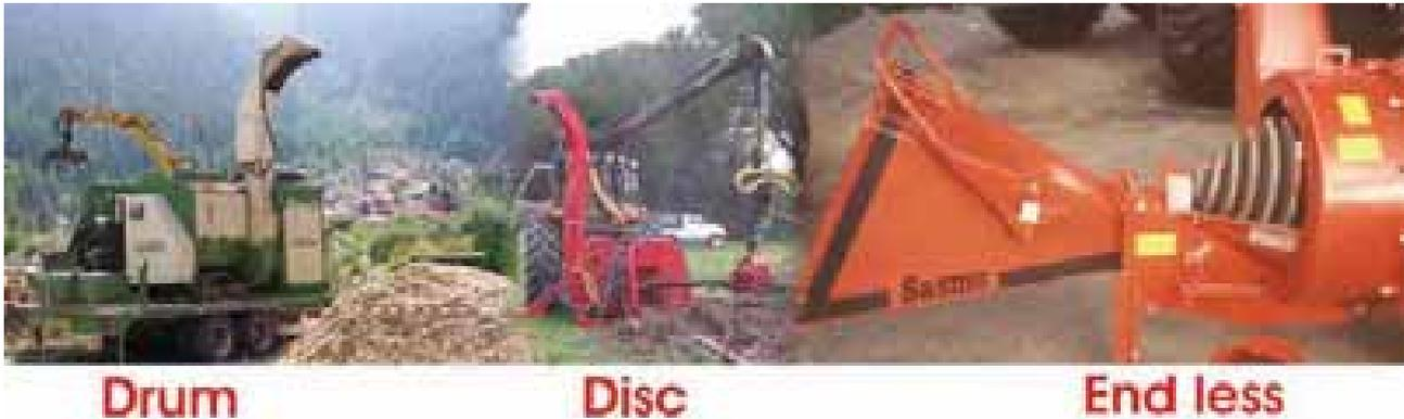
Photo 30. Three different types of chippers based on cutting element.
