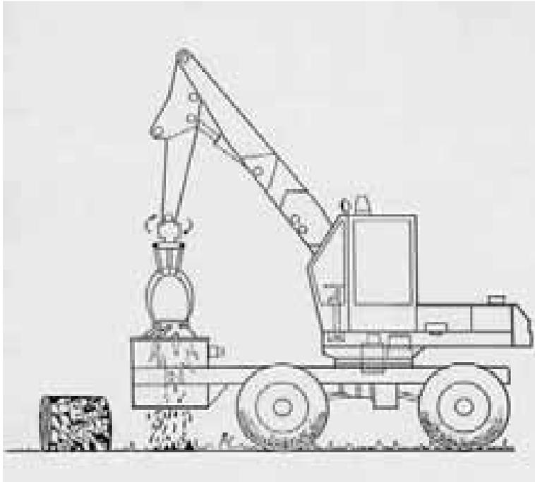
Figure 12. As an alternative the cleaner can be mounted directly on the chassis of the loader, resulting in a more compact and agile unit.
