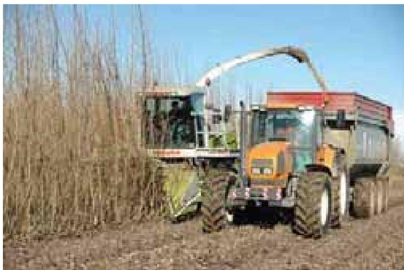
Photo 45. The tractor moves by the side of the harvester, when the trailer is full it unloads the chips at the landing while the forager fills a second tractor
