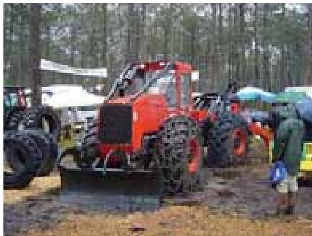
Photo 24. Articulated forest tractor fitted with a grapple (grapple skidder).
