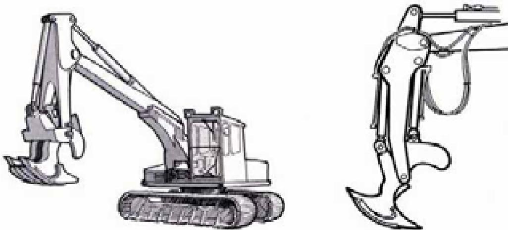
Figure 10. The *Pallari* grapple mounted on an excavator and a profile detail of the attachment.
