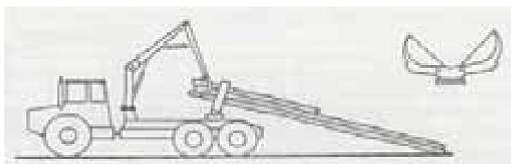
Figure 9. Tractor equipped with a clam bunk.
