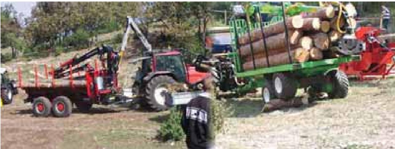
Photo 21. Forest trailers with hydraulic knuckle-boom loader.
