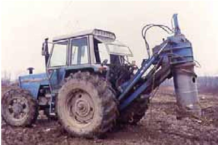
Photo 33. The auger type extractor is basically a cylinder large enough to contain the taproot of a mature poplar
