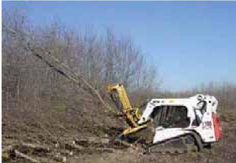
Photo 56. A mini feller buncher can handle up to two whole trees per work cycle.
