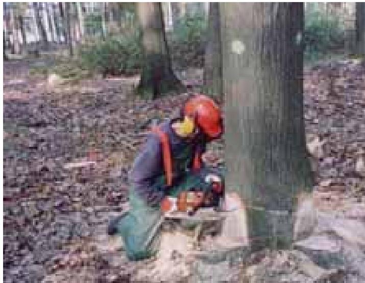
Photo 6. Chainsaw operator while he makes an undercut, equipped with suitable gear for individual protection.
