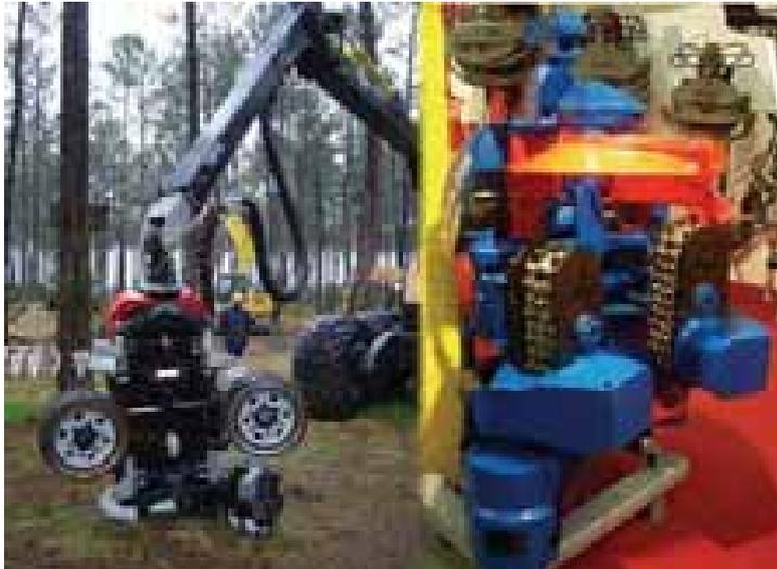
Photo 8. Two models of felling heads and processors. The cutting element is a grooved bar along which a cutting chain runs.
