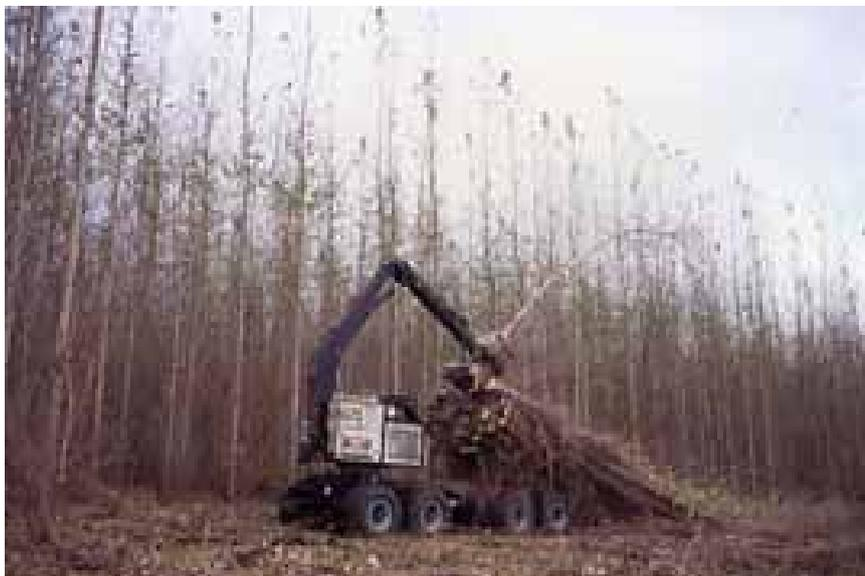
Photo 49. As an alternative to the excavator, a dedicated prime mover can be used. The shown model harvests the trees and collects them in the rear clam bunk.
