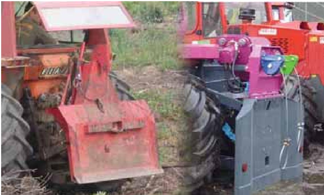
Photo 17. On the left a mobile forestry winch; on the right a fixed mobile winch.
