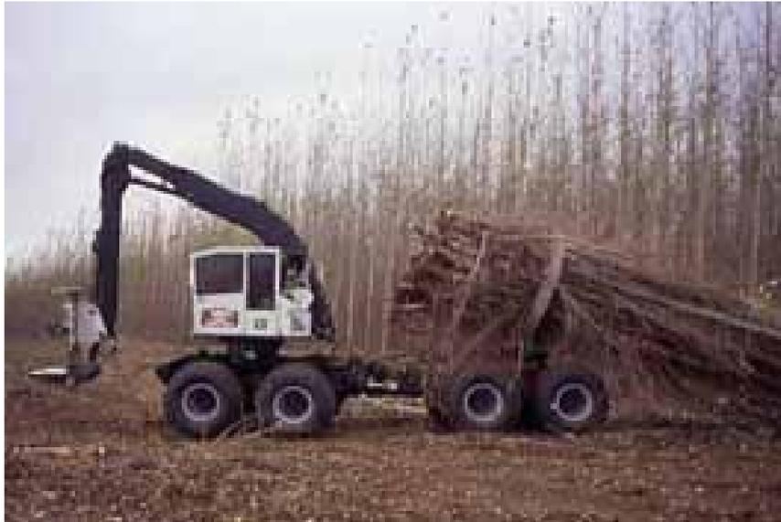
Photo 50. When the load is complete the feller moves by the side and leaves the bunch of trees ready for forwarding.
