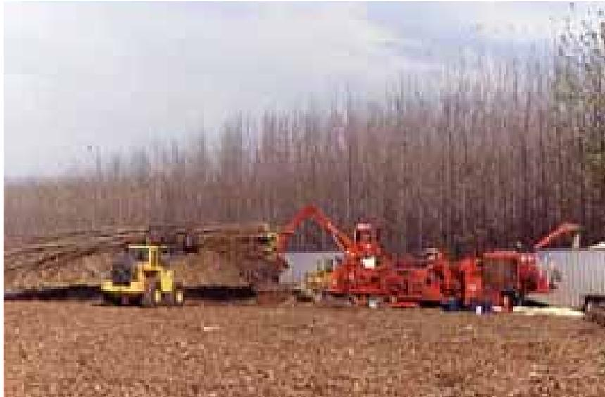
Photo 52. At the landing the mobile Delimber-Debarker-Chipper loads directly the trailers.
