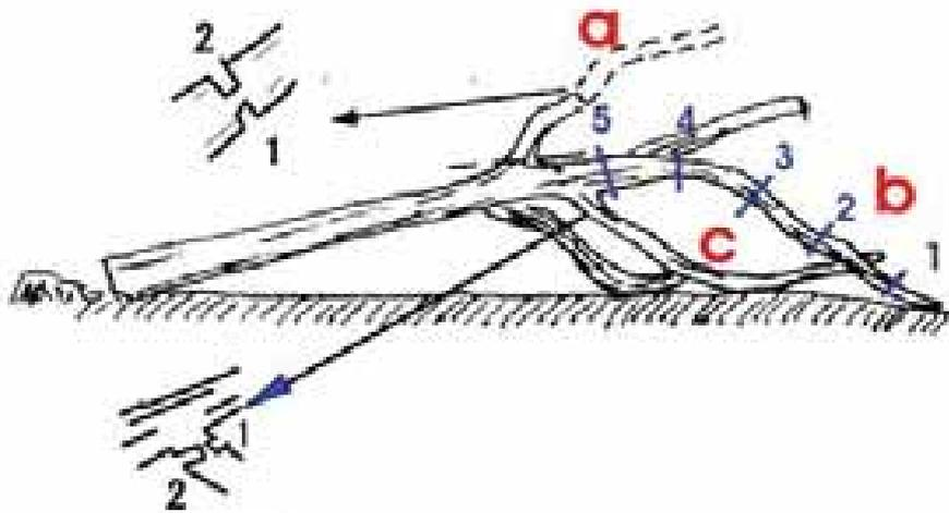
Figure 2. Correct method for delimiting hardwood trees.
