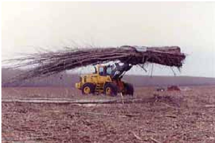
Photo 51. A powerful front-end loader transports the bunch of whole trees to the landing.
