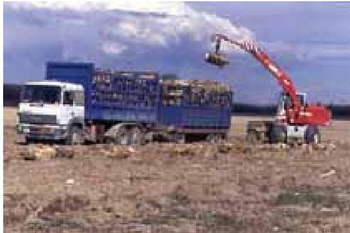
Photo 38. Common truck and trailers can enter directly into the field when the soil is dry, the loader can quickly fill these units reducing their expensive waiting time.
