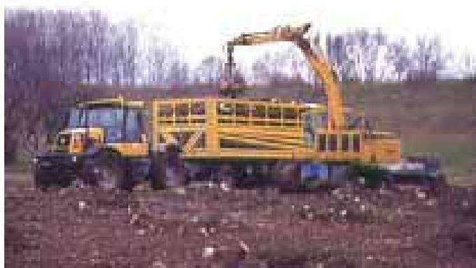
Photo 39. High speed tractors with 3 axes trailers may provide a good compromise between cross-country mobility and road speed.
