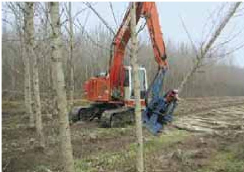
Photo 57. An excavator based harvester can harvest and process the trees accumulating tops and logs in different heaps or rows.
