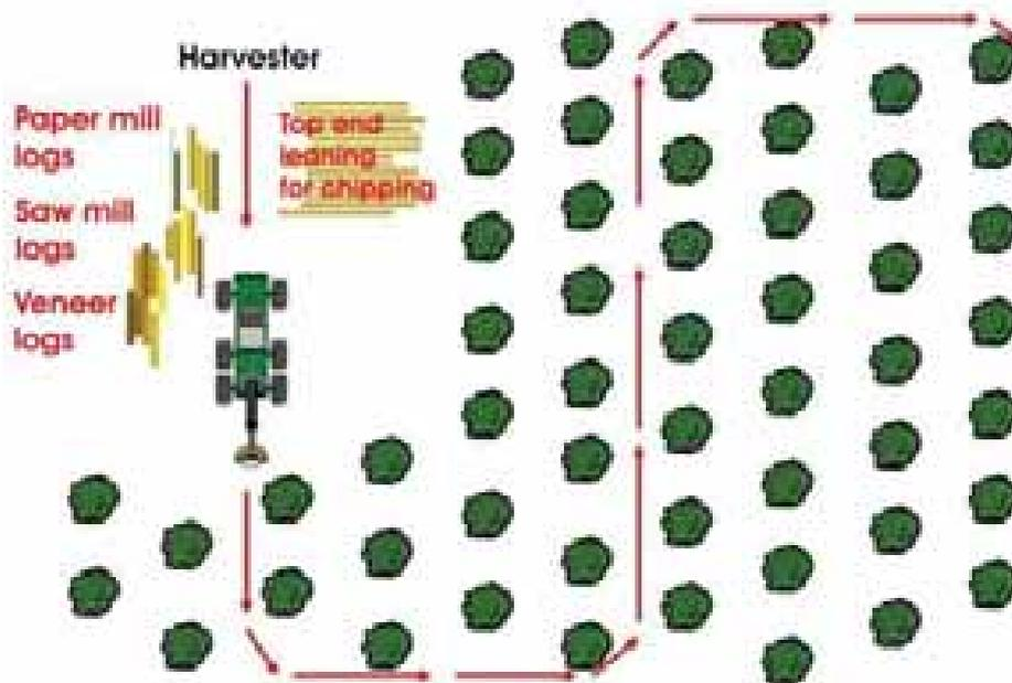
Figure 6. Rational operational scheme of using full mechanization in poplar logging.
