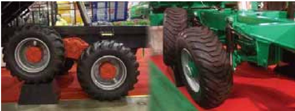
Photo 20. On the left equalizer axle system with hydraulic traction; on the right hydraulic system for steering and levelling the trailer axles.
