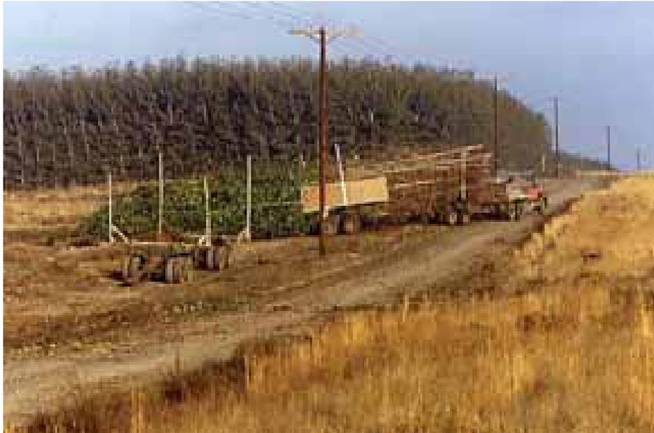
Photo 53. At the roadside the full trailers are transferred to trucks for road transportation to the central landing.
