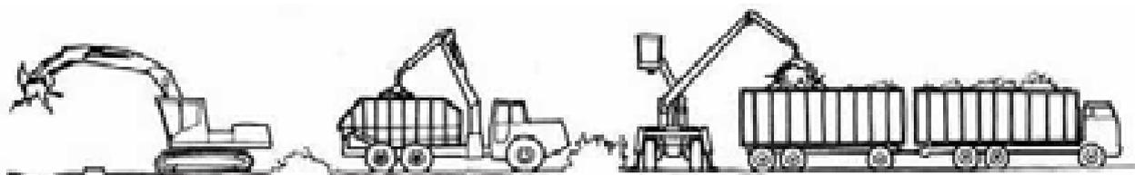
Figure 11. Root extraction system based on *Pallari* grapple; roots are leaved in the field outdoors for a few months to allow the rain to wash soil out.
