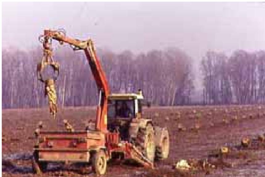
Photo 35. A common farm tractor may operate the cleaner, but it requires an additional pump to operate it together with the crane.
